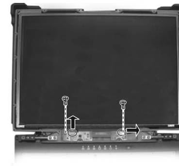
Figure 2-18 Remove two screws and disconnect two cable
